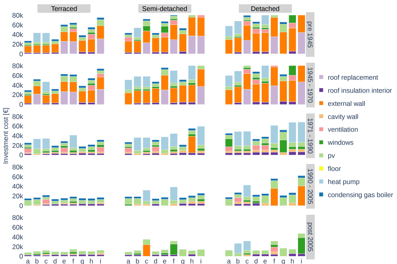
Figure 13: The OPEX optimized renovation packages of the building archetypes. Note that, for the purpose of comparison with [3], and unlike the discussion following Figures 4 and 5, the results have not been scaled to their relative occurrence in the Flemish building stock.
