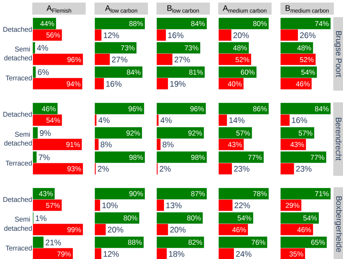
Figure 21: Overview of TCO - optimized choice of heating system for the carbon scenarios for the districts Brugse Poort (Ghent), Berendrecht (Antwerp), and Boxbergerheide (Genk).
