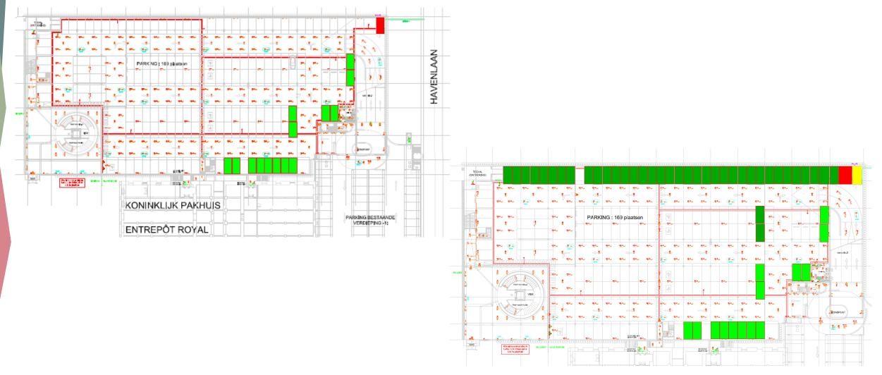
Future EV-installation in Parking Esplanade: 54 charging points on a 1.000kVA transformer
