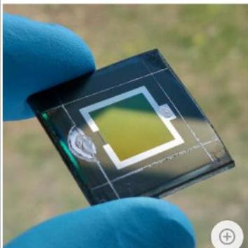
A special branch in the famous NREL-chart for solar cell world records refers to a newly developed tandem solar cell by HZB teams. The world-record cell combines the semiconductors perovskite and CIGS to a monolithic "two-terminal" tandem cell. Due to the thin-film technologies used, such tandem cells survive much longer in space and can even be produced on flexible films. The new tandem cell achieves a certified efficiency of 24.16 percent.
