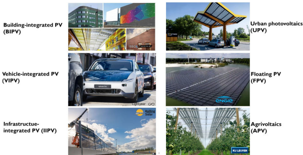
Figure 2: Various types of integrated PV. Within SolarEMR we target BIPV with a façade application and IIPV with a noise barrier application. Source picture: IMEC.
