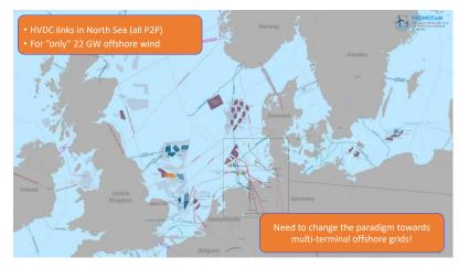
HVDC is key technology for large-scale integration of renewable energy sources
