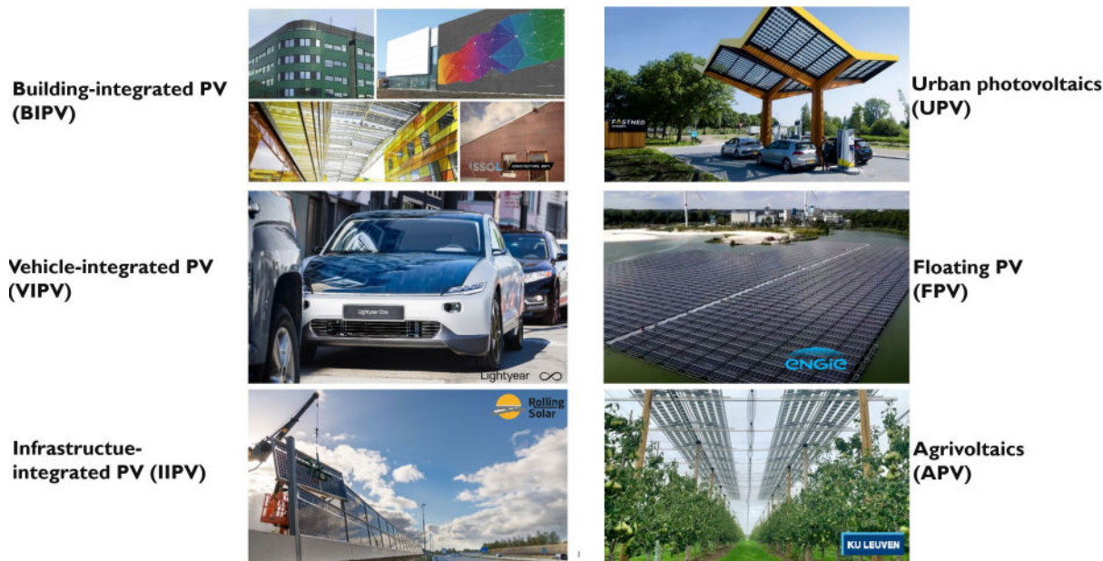
Figure 2: Various types of integrated PV. Within SolarEMR we target BIPV with a façade application and IIPV with a noise barrier application. Source picture: IMEC.
