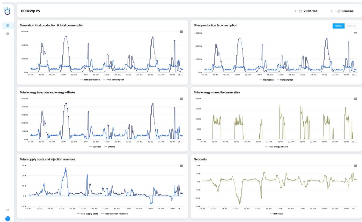
Figure 11: Visual representation of the 600 kWp noise-barrier IPV installation + energy sharing simulation of the tunnel for a given week
