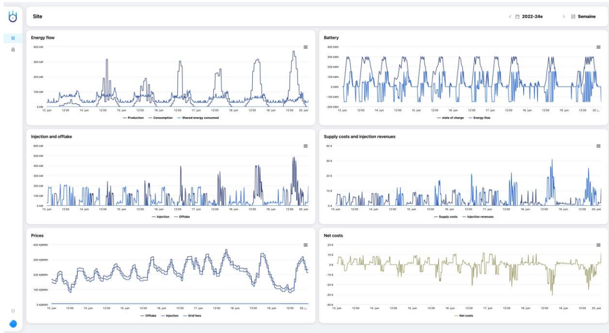
Figure 7: Visual representation of the energy flows and prices for the 600 kWp noise-barrier IPV installation + 300 kWh battery simulation for a given week
