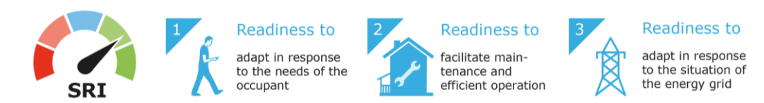
Figure 2 – Three key functionalities of smart readiness in buildings
