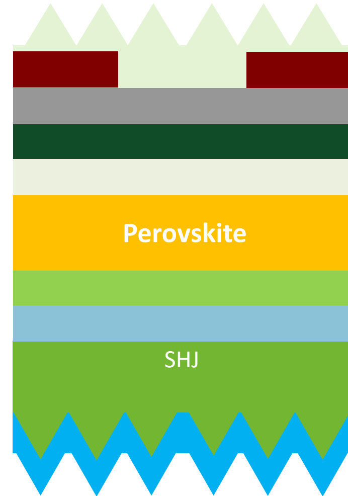
Frontside polished Si cell Textured front structure added
